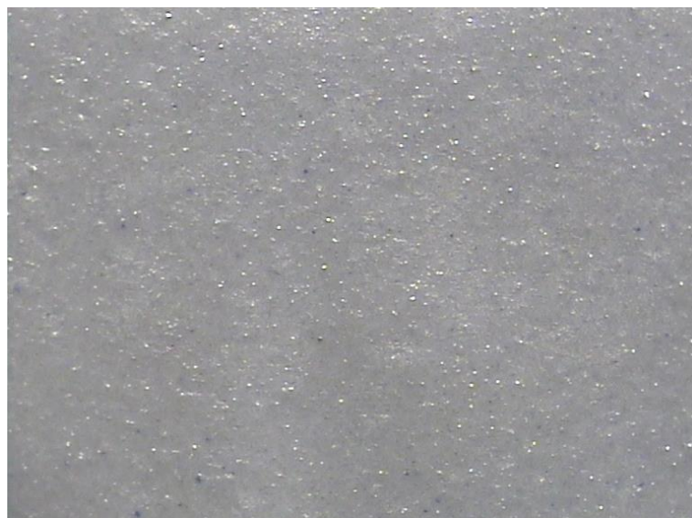
Photo 2: Material Teroson MS 937, color grey (at a magnification of x 50) after an incubation period of 28 days without fungal growth
